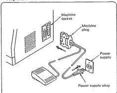
NOTE: Before inserting the plug into your machine, be sure the power switch is OFF.
